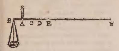
Suppose an equal weight at C, unto that at B, (which points are both equally distant from the center A,) it is evident that then the beam BF, will hang horizontally. But if the weight supposed at C, be unequall to that at B, or if there be an equal weight at DE, or any of the other unequal distances; the Beam must then necessarily decline.
